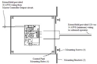
**Wiring the Remote Operator:** This unit is not provided with a power supply. Only connect 24-vac from an approved source at the input terminals on the pc board. Connect 24-vac cable from Master Controller as shown. For Units operating 120-vac devices, 120-vac line should be routed from power source through terminals as shown. Neutral can be routed separate from the wiring at this unit. Extend 24-vac to device as shown where the control is 24-vac.
